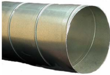
GALVANIZED SPIRAL PIPE GP01 XXZZ XX= DIAMETER 03-36 ZZ=GAUGE 22, 24, 26 SPECIFY SMOOTH OR RAISED BEAD STANDARD LENGTH IS 10' OR 20' $2/CUT CHARGE FOR ALL OTHER SIZES
