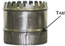
417 COLLAR LONG EXT. W/TABS RX14 XX XX=04-28" TABS KEEP FLEX FROM SLIPPING OFF COLLAR
