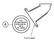
This gasket **must** be used on the Flat Flange Heads.
