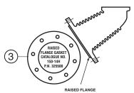
This new gasket, specifically designed for the Raised Flange Heads, may be used.
