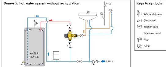
\*MixCal<sup>™</sup> 521 series thermostatic mixing valves with inlet check valves, "AC" models, can be used instead of separately installed check valves.
