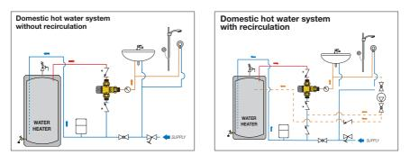
\*MixCal series 521 thermostatic mixing valves with inlet check valves, "AC" models, can be used instead of separately installed check valves.
