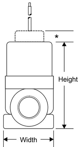
\* For valves with a conduit hub at the top, add 0.44 in. (11 mm) to the height dimension.
