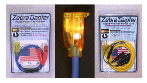
Zebra'Dapters are a significantly **SAFER** way to obtain and use 120 Volt power when performing service. **Safer** because positive power indication is provided via a light in the end of the cordset; it indicates whether or not 120 Volt power is present an the connection point (and, in Model ZD002, also indicates if power is accidently tapped from a 208/240 volt source instead of the desired 120 volts). Also, they're safer because the hot line is fused to help prevent 'accidents' while working.
