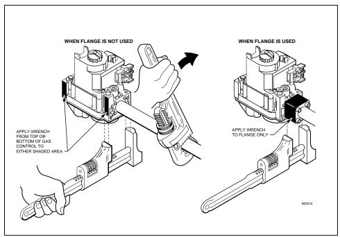
FIG. 5—PROPER USE OF WRENCH ON GAS CONTROL WITH AND WITHOUT FLANGES.
