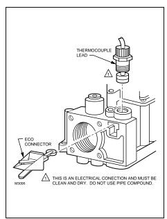
FIG. 7—INSTALLING THERMOCOUPLE AND OP-TIONAL ECO ADAPTER TO THE POWER UNIT.
