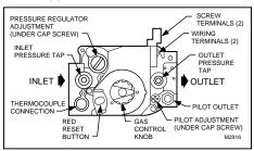
FIG. 4—TOP VIEW OF GAS CONTROL.
