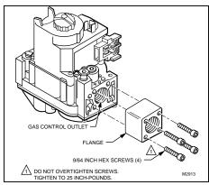
FIG. 1—FASTEN FLANGE TO VALVE WITH 25 INCH-POUNDS TORQUE.
