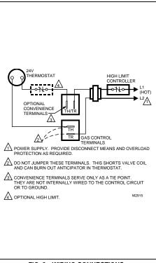
FIG. 8-WIRING CONNECTIONS.
