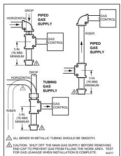
FIG. 2—SEDIMENT TRAP INSTALLATION.
