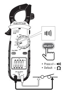
Buzzer sounds at less than  $40\Omega$ .
