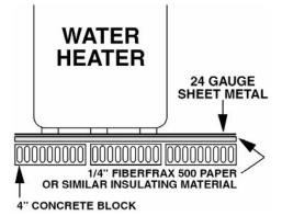
Minimum clearance to combustible construction is: SIDES 6"; BACK 6"; FRONT 24". The installation of this water heater must conform with local codes and ordinances. In the absence of local codes, the installation must comply with the National Fire Protection Association (NFPA 31) Code.
