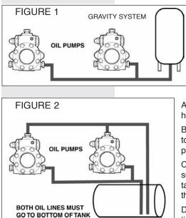
3. Return lines must be the same diameter as suction lines and extend close to the bottom of storage tank but stop slightly above suction lines. Use a minimum of fittings and make bends in tubing with as large a radius as possible. Always use flared fittings, not compression fittings. If pipe is used instead of tubing, do not connect the burner to the pipe – use copper tubing and form a coil before attaching tubing to burner.
