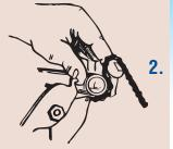
Holding the cutter in the opposite hand with the handles in the open position, guide the cutter chain around the tubing at the point where the cut is to be made.
