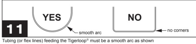
**11** Tubing (or flex lines) feeding the Tigerloop® must be a smooth arc as shown
