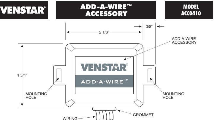
Fig.1 - ADD-A-WIRE <sup>™</sup> Accessory Mounting
