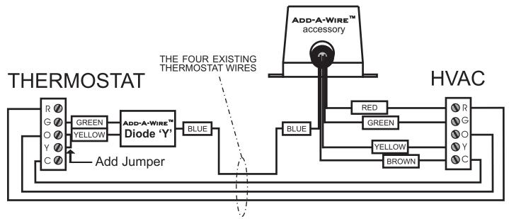
4 existing wires with ADD-A-WIRE™ to accommodate a single stage heat pump. A jumper is required across the 'Y' and 'O' thermostat terminals.
