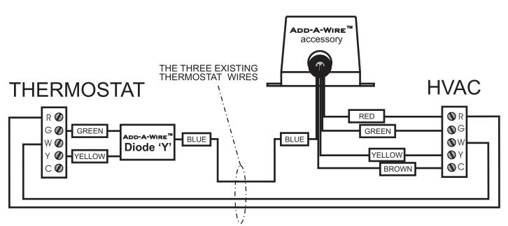
3 existing wires with ADD-A-WIRE<sup>™</sup> to add a cooling to a system that already has heating.
