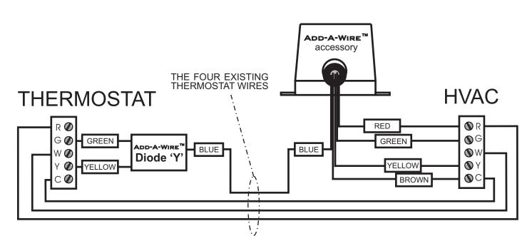
4 existing wires with ADD-A-WIRE™ to accommodate a thermostat that requires 5 wires.
