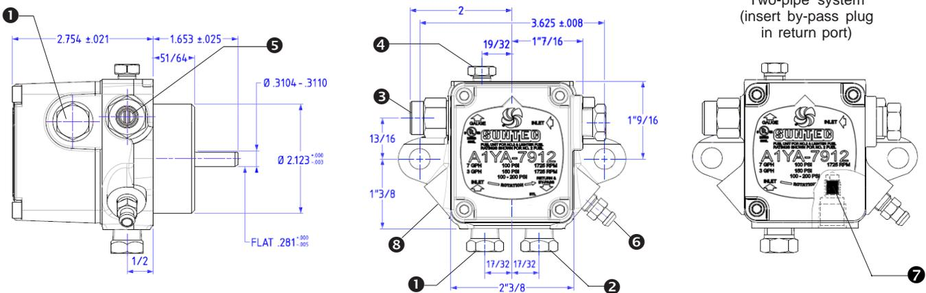
① Inlet ② Return ③ Nozzle outlet ④ Pressure gauge port ⑤ Pressure adjustment ⑥ Bleeder valve ⑦ Internal by-pass plug ⑧ Cone valve
