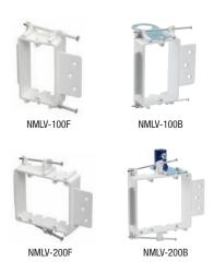
NMLV-100F and NMLV-200F used on 3/4" thick furring strips, 2" x 4" wood or steel stud. Provided with 2 nails for use on 2" x 4" wood stud. Use No. 6 flat head screws for steel stud or 3/4" thick furring strip. NMLV-100B and NMLV-200B used on 2" x 4" wood or steel stud with 1/2" or 3/4" EMT. Provided with 2 nails for use on 2" x 4" wood stud. Use No. 6 flat head screws for steel stud. Steel bracket will accommodate 1/2" or 3/4" EMT connector. Patented.
