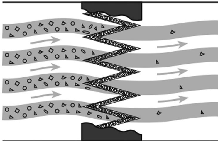
**Skuttle's superior depth-loading filter design captures more airborne particles and lasts longer than many common filter media.**
