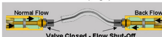
Hose Failure - Hose Separation
