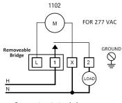
For separate motor terminals remove bridge from terminal L & 1.
