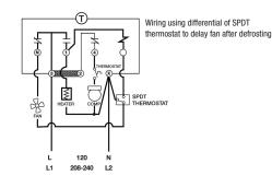
Models 8245-00 and 8245-20 -Wiring Diagram
