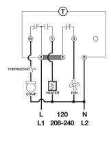
Fan and compressor loads not to exceed 2 hp. Heater not to exceed 4000 watts at 120V AC or 8000 watts at 240V AC
