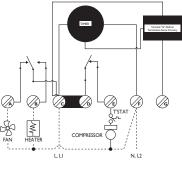
9145 ELECTRIC DEFROST - Time Initiated Time Terminated - Wiring Diagram
