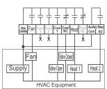
Sw 1 = Off - HE (Fan on With Heat) Sw 2 = On - HC (Heat/Cool) Aux Relay Mode = Aux Heat
