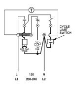
Wiring using 120V or 240V single phase line with compressor thermostat closed during defrost.
