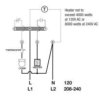
Models 8041-00 and 8041-20 - Wiring Diagram
