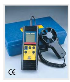
This hand-held instrument reads both air velocity and temperature simultaneously when balancing air conditioning/heating ventilation systems.
