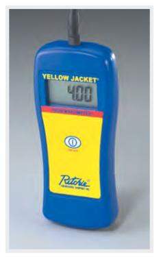
The digital electronic manometer eliminates the mess and fragility of U-tubes or diaphragm type gas pressure gauges. This easy-to-use instrument provides a continuous display of the measured positive or negative pressure. Ideal for setting gas pressure at manifold, checking pressure, flue draft and air balancing. Kit includes battery, 18" tubing and brass fitting.
