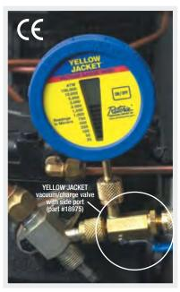
Connect to the YELLOW JACKET SUPEREVACT Vacuum Pump, in line with a tee fitting or directly to the system with YELLOW JACKET core removal tool 18975.
