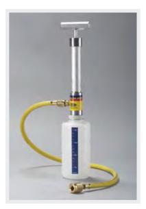
Self-contained injection system for inducing up to 16 oz. of universal AC/R dye into the largest systems. Add to the lo-side. Easily works on all system pressures to 300 psi, .35 oz. per stroke. Hose included with SealRight end.
