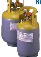
These gray and yellow 30 and 50 lb. cylinders feature "Y" valve for liquid/vapor, 400 psi rating and 3/4" plug for a float switch.
