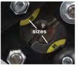
2. Select sizes on underside of dies to match tubing
