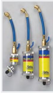
Body and cap are rugged aluminum with an "O" ring seal. 1/4" Male fitting at one end with Schrader, A ball valve for control on other end with a short length of hose. Valve depressor in 1/4" Female end. 600 psi working pressure.
