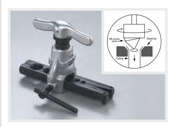
Off-center hardened steel cone with 45° flare produces a rolling action for uniform flare walls without galling in 3/16" to 3/4" O.D. tubing.
