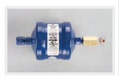
High capacity in-line filter drier removes moisture and oil breakdown products, as well as acid from burnt out systems. Attaches directly to refrigerant recovery system with a 1/4" female and a 1/4" male connection. UL and CSA listed.
