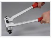
With long handles for comfortable leverage, easily expand 5/16" to 1-5/8" O.D. soft copper and aluminum tubing in seconds. Select from nine expander heads to attach to the front of the handles.
