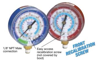
Housed in a red or blue steel case for durability. Colored temperature scales are easy to read through polycarbonate crystal. Several features combine for improved accuracy: Flutterless™ technology with brass surge protector to minimize needle pulsation, brass gauge
