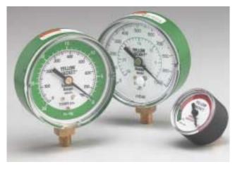
Full range mechanical bourdon tube gauges for determining system vacuum. Much more accurate than a compound gauge. All gauges are 1/8" NPT Male bottom connection.
