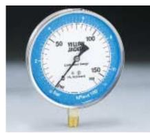
Large 4-1/2" dial for easy reading. Stainless steel case. Brass movement and 1/4" NPT Male socket bottom mount. Gauge has recalibrator screw. A surge protector to help dampen needle pulsation. 1% accuracy (Class 1) calibration full scale.
