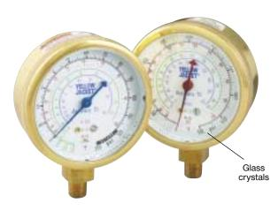
Solid brass case and premium movements. Heavy duty phosphor bronze and stainless steel internal components for longer service life under severe use. 1% accuracy (Class 1) calibration. Flutterless<sup>™</sup> technology with brass surge protector to minimize needle pulsation.
