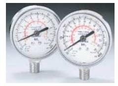
Ammonia gauges are designed for use on manifolds and as permanent gauges on any system or equipment charged with ammonia. The bourdon tube is made of 316 stainless. The sockets are steel. The dials show dual temperature and pressure scales. All gauges are equipped with restrictors to protect the gauges against pulsating pressure. Steel gauge cases are painted black. Gauges calibrated to 3-2-3% accuracy.
