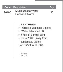
**Application** • The AquaGuard AG-9150E is the ultimate condensate management system for any residential or commercial application. The AG-9150E features our award winning AG-1250E Multipurpose Water Sensor combined with our AG-9100 External Audible and Visual Remote Alarm. For metal or plastic secondary pan, floors, walls and basement installations.
