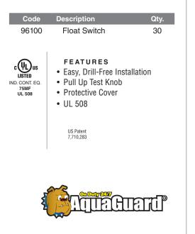
**Application** • The AG-1100+ is incredibly easy to install. It can be mounted to the drain pan in 10 seconds or less. Installation does not require any pre-drilling for screws. The AG-1100+ incorporates a protective cover to keep out insulation and debris that could prevent the float from rising.
