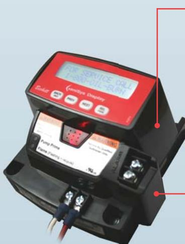
**The GeniSys Display (Pt. No. 52067)** allows a technician to monitor and program the primary control variables. The display shows current burner status, control timings, and burner cycle history. The display's programming mode allows a technician to customize both the pre-time and post-time settings and a lockout service message.
