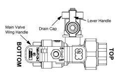
Figure 1. Valve Detail (Cold Water Valve shown)
