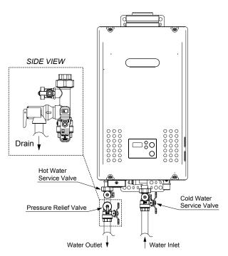
Figure 2. Completed Installation
