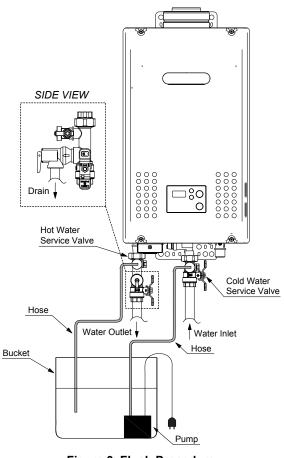
Figure 3. Flush Procedure
