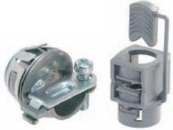
A concern with two cable usage is the fitting's ability to withstand cable pullout forces normally encountered during installation. Per UL 514B, each cable is subjected to an individual pull test. In addition, UL tests strap type connectors to ensure that when tightening the strap screws, the strap will not pierce the nonmetallic sheath of the cable, creating a possible short.
