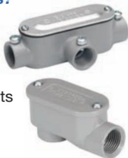
Conduit bodies provide access to the conduit system through a removable cover at a junction of two or more entries. Bodies may be used for changing the direction of the wiring systems, to aid in pulling of long wire runs, or to mount devices or make splices.
