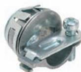
For connecting nonmetallic cable to box or enclosure. Also listed for use with SJO cord. Simply snap connector into electrical box. External spring steel locking tabs secures connector to electrical box. Patented Whipper-Snap design.
