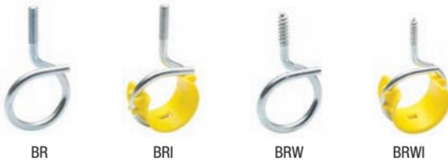
Steel bridle rings provide support for voice, data, or video cables. Open loop end allows easy insertion of cables. Machine thread style for use with beam clamps or other clamping devices. Wood style rings are threaded for easy assembly into pre-drilled holes.
