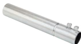
Assembles like a regular Rigid/IMC set screw coupling. To install, simply slide coupling end stop onto fixed end of conduit and tighten set screw. Place movable conduit end completely into coupling and mark engagement, remove conduit and mark half the distance of engagement, reinstall conduit to half the distance. Bonding jumper purchased separately. US Patent 6,715,803B1.
