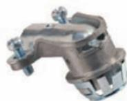
Used for connecting AC/MC cable or flexible metal conduit to box or enclosure. Simply snap connector into electrical box. External spring steel locking tabs secures connector to electrical box. Patented Whipper-Snap design.
