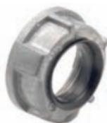
Used with locknut to protect conductors inside threaded rigid or IMC conduit entering a box. Plastic liner prevents damage to wire insulation. All products rated 150°C except catalog numbers 371 and 372 which are rated 105°C.
