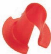
When installing ARMORED CABLE (Type AC), NEC Article 320 mandates the use of a insulating bushing (commonly referred to as Anti-Short or Redhead) between the metal sheath and the conductors. Fittings with insulated throats are not a substitute for the anti-short bushing.
