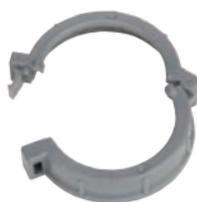
Patented split design allows for installation after conductors have been pulled. Used with a locknut to terminate threaded rigid and IMC to a box or enclosure. Used with a connector to prevent damage to wire insulation. Rated 105°C.
