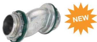
Bridgeport's raintight offset nipples are used to offset the axis of a raceway 3/4" between enclosure runs. Rugged zinc die cast construction ensures mechanical protection and durability. Integrated sealing washers maintain wet location/raintight seal. Completely assembled with locknuts and sealing washers. Patented.
