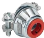
For connecting AC/MC cable to box or enclosure. CSA Listed for ACG90. Refer to the cable connector compatibility charts in the technical guide section for MCI-A and other cables. Connector simply snaps into the box. Patented Whipper-Snap design.
