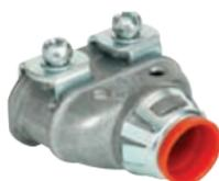
For connecting flexible metal conduit to box or enclosure. Connectors simply snap into the electrical box. Suitable for maintaining grounding continuity when installed in accordance with the NEC. Also see AC/MC section for additional listings. Patented Whipper-Snap design.
