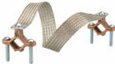
Use Bonding Jumper Assembly to comply with Article 250 of the National Electrical Code. Suitable for use on EMT, rigid conduit, or copper water pipe. If used with expansion coupling: assemble ground clamp to conduit one inch from stationary end of coupling. Attach second ground clamp two inches from sliding end of expansion coupling. Assembly features bronze ground clamps and copper bonding strip.
