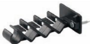
NMCB-2 is provided with a nail for use on wood studs or 3/4" thick furring strips to position nonmetallic sheath cable. Capable of positioning nonmetallic cables in each of three rectangular slots. May also be used with low voltage cable. Low profile design and unique self-locking fingers prevent accidental removal of cables. Grooved nail for extra gripping with stud. Patented.
