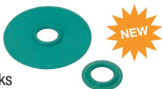
Used when a concentric knockout breaks out larger than expected. Maintains NEMA 3R rating on listed enclosures. Includes one coated and one uncoated washer. Coated washer installs on the exterior of the box. Sunlight resistant. Patent Pending.
