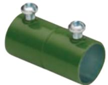
Set screw coupling used to join two lengths of EMT. Color coded green to match EMT for easy identification. Use with green EMT for critical circuits, nurse call stations and hospital and healthcare applications. Concrete-tight. Furnished with Tri-Drive slot/Phillips/Robertson head screws. Patented.
