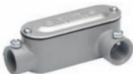
Units have a threaded interior for use with rigid or IMC as well as set screws for use with EMT. Preassembled with cover and gasket.
