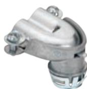
90° fitting with steel cover used to connect AC/MC or flexible metal conduit to box or enclosure. Simply snap connector into electrical box! External spring steel locking tabs secures connector. Refer to the cable connector compatibility charts in the technical guide section for MCI-A and other cables. Patented Whipper-Snap design.
