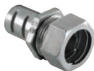
Coupling used to join EMT to flexible metal conduit. Screw-in end for flex. Compression end for EMT.
