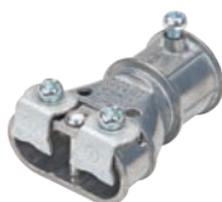
Coupling used to join duplex flexible metal conduit to EMT. Set screw type transitional fitting ideal for commercial and institutional facilities. A labor savings, compared to the traditional junction box installation. Simply remove the armor and expose the length of conductors to reach the device box or enclosure. Insert FMC or AC/MC until visible in inspection holes. Also see AC/MC section for additional listings. Patented.
