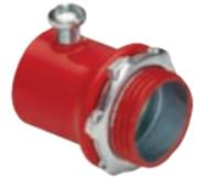
Set screw connector used to join EMT to box or enclosure. Color coded red to match EMT for easy identification. Use with red EMT for emergency circuits, fire alarm and security system applications. Concrete-tight. Furnished with Tri-Drive slot/Phillips/Robertson head screws. Patented.
