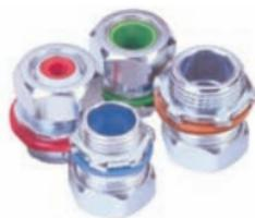
Bridgeport's line of high quality, made in the USA, cord grip fittings is the electrician's smart choice. Each fitting is identified by a color coded grommet that clearly indicates the minimum-maximum cable diameter range for which the connector can be used. Bridgeport's cord grips meet the requirements of
