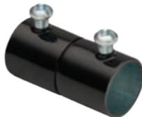
Set screw coupling used to join two lengths of EMT. Color coded black to match EMT for easy identification. Use with black EMT in dark colored areas or in open architecture applications. Concrete-tight. Furnished with Tri-Drive slot/Phillips/Robertson head screws. Patented.
