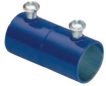
Set screw coupling used to join two lengths of EMT. Color coded blue to match EMT for easy identification. Use with blue EMT for low voltage wiring, data comm/video and network security applications. Concrete-tight. Furnished with Tri-Drive slot/Phillips/Robertson head screws. Patented.
