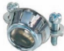
For connecting nonmetallic cable to box or enclosure. Simply snap connector into electrical box. External spring steel locking tabs secures connector to electrical box. Patented Whipper-Snap design.
