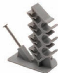
For use on steel or wood studs to support nonmetallic sheath, communication, and data cables. Furnished with nail for wood stud. Use No. 8 x 1/2" self-tapping sheet metal screw for steel stud. Complies with NEC Articles 300-4(D) and 320.23(B). Patented.
