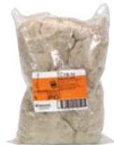
Fiber is used to separate conductors from each other and from the sealing compound. The fiber then forms a dam within the sealing fittings that allows the poured sealing compound to harden in place.
