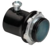
Set screw connector used to join EMT to box or enclosure. Color coded black to match EMT for easy identification. Use with black EMT in dark colored areas or in open architecture applications. Concrete-tight. Furnished with Tri-Drive slot/Phillips/Robertson head screws. Patented.
