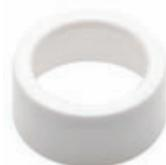
EMT bushing insulates telephone, computer, video and other low voltage wiring from sharp edges of EMT. Complies with NEC Article 300-15(c).
