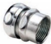
Used to join rigid or IMC to EMT. Coupling internally threaded for rigid / IMC. Compression type for EMT. Concrete-tight.
