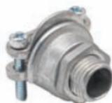
Used to connect nonmetallic sheath cable (NM-B), AC/MC cable or flexible metal conduit to 1/4" knockout. Will fit 1/4" knockouts with flats, such as used in lighting applications.
