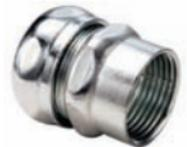
Coupling used to join EMT to rigid or IMC. Coupling internally threaded for rigid / IMC. Compression type for EMT. Concrete-tight.
