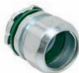
Compression type connector with internal sealing ring and knockout gasket to create a raintight seal when connecting EMT to box or enclosure.
