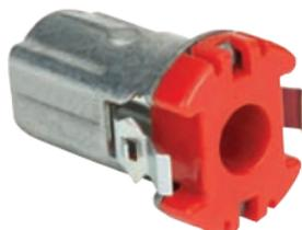
Pull cable into box, snap cable into connector and snap connector into box. No tools required! Refer to the technical guide section for MCI-A and other cables.
