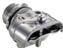
Strap type fitting used to connect nonmetallic cable, flexible metal conduit and AC/MC cables to box or enclosure. CSA Listed for ACG90. Refer to the cable connector compatibility charts in the technical guide section.
