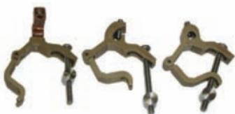
Designed for the grounding and bonding of electrical and plumbing systems. The SDB series are constructed of bronze and assembled with stainless steel hardware and are available in three distinct styles: lay-in lug, copper lug and enclosed style. The SDB series are listed for attachment to EMT, rigid conduit raceways and steel and copper water piping systems. Patent Pending.
