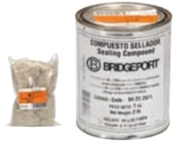
Fiber is used to separate conductors from each other and from the sealing compound. The fiber then forms a dam within the sealing fittings that allows the poured sealing compound to harden in place. The sealing compound provides a seal between and around the conductors within the fittings. UL Listed for use with Bridgeport **EYS** and **EYS-N** series sealing fittings.
