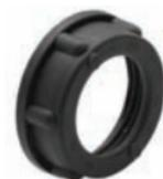
Used with locknut to protect conductors inside threaded rigid or IMC conduit entering a box. Rounded surface of bushing prevents damage to wire insulation.
