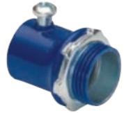
Set screw connector used to join EMT to box or enclosure. Color coded blue to match EMT for easy identification. Use with blue EMT for low voltage wiring, data comm/video and network security applications. Concrete-tight. Furnished with Tri-Drive slot/Phillips/Robertson head screws. Patented.
