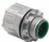
To secure threaded rigid service entrance conduit to box or enclosure. Insulated throat rated 105°C. BUNA-N sealing ring completely encircles knockout to prevent contaminants from entering enclosure. Concrete-tight.
