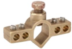
Ground Rod Bridge Clamps used as an intersystem bonding means by utilizing 4-terminal points for connecting communication systems to the same electrical grounding electrode/rod. Meets the requirement of NEC Article 250.94. Direct Burial Rated. Patented.
