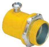
Set screw connector used to join EMT. to box or enclosure. Color coded yellow to match EMT for easy identification. Use with yellow EMT in special equipment, caution areas, and high voltage applications. Concrete-tight. Furnished with Tri-Drive slot/Phillips/Robertson head screws. Patented.
