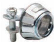
For connecting SJO cord to box or enclosure. Also listed for NM-B cable - see Nonmetallic Cable section. Simply snap connector into electrical box. External spring steel locking tabs secures connector to electrical box. Patented Whipper-Snap design.
