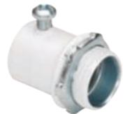
Set screw connector used to join EMT to box or enclosure. Color coded white to match EMT for easy identification. Use with white EMT in light colored areas and open architecture applications. Concrete-tight. Furnished with Tri-Drive slot/Phillips/Robertson head screws. Patented.
