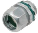
Compression style connector with internal sealing ring and knockout gasket to create a raintight seal when connecting EMT to box or enclosure. Patented.
