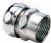
Used to join rigid or IMC to EMT. Coupling internally threaded for rigid / IMC. Compression end for EMT. Concrete-tight.
