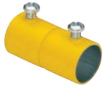
Set screw coupling used to join two lengths of EMT. Color coded yellow to match EMT for easy identification. Use with yellow EMT in special equipment, caution areas, and high voltage applications. Concrete-tight. Furnished with Tri-Drive slot/Phillips/Robertson head screws. Patented.
