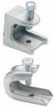
UL Listed Beam Clamps are manufactured from malleable iron or steel with a hardened screw to secure the clamp to the beam. Clamps are tapped in two places for attachment of threaded rod, conduit hanger, or bridle ring.
