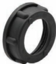
Plastic insulating bushings must be used in conjunction with two locknuts when connecting threaded rigid or IMC conduit, containing No. 4 or larger un-grounded conductors, to boxes or enclosures.
