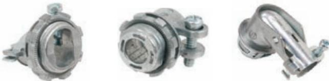
NEC Article 300.15 specifies that fittings can only be used with wiring methods for which they are designed and listed. Most manufacturers have received dual usage listings for these types of connectors; however, you should not assume all fittings have the dual listing. While the appearance of Metal Clad (MC) and Armored Cable (AC) connectors may be similar, the misuse of an AC cable connector can be significant enough to cause an unsafe installation with metal clad cable.
