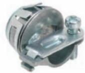
For connecting nonmetallic cable to box or enclosure. Also listed for use with SJO cord. Simply snap connector into electrical box. External spring steel locking tabs secures connector to electrical box. Patented Whipper-Snap design.
