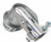
90° fitting with cover used for connecting AC/MC cable to box or enclosure. Single screw design saves time and money. Connectors with patented Whipper-Snap design snap into electrical box! Concrete-tight when taped. Refer to the cable connector compatibility charts in the technical guide section for MCI-A and other cables.
