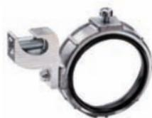
Used with locknut to terminate service conduit to cabinet. Aluminum alloy lug provided for bonding jumper to neutral busbar. Plastic liner prevents damage to wire insulation.
