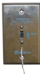
Provides for emergency call activation by pulling the supplied nylon cord downward. The call is reset at the station by simply pushing the activation switch upward. The station mounts in a standard single gang box. The units' stainless steel faceplate is marked "Emergency Pull For Help". 6 amps at 125VAC. DPST Switch.
