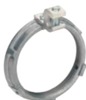
Used to fasten threaded connectors or nipples to box or enclosure. Offers an additional bonding/grounding path. Listed for use with rigid conduit, threaded hubs and conduit nipples.
