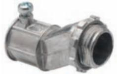
Set screw type connector used to join EMT to box or enclosure. Concrete-tight. 1620-DC2 has 3/8" offset; 1621-DC2 has 3/4" offset.
