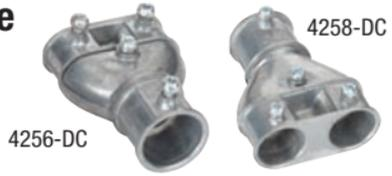
Used to join two lengths of EMT conduit into one. The 4256-DC joins two 1/2" EMT to one 3/4" EMT. The 4258-DC joins two 3/4" EMT to one 1" EMT. Patented.
