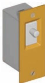
All purpose electric door switches for use anywhere that lights are turned on and off automatically by the opening and closing of a door. Units may be wired either normally open or normally closed. The units are shipped normally closed. The switch mounts using the 3" (76mm) on center mounting holes.
