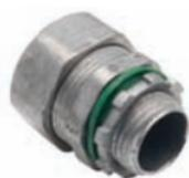
Straight connector for use with any flexible cord. Provides liquid tight, watertight protection. Tapered (NPT) threads. Furnished with polyethylene knockout gasket and locknut.
