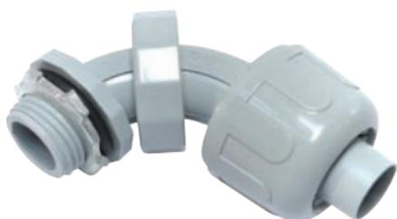
Push-on, multi-angle connectors for nonmetallic "Type B" liquid tight conduit. Simply push the connector into the conduit and tighten the domed sealing nut. Molded of Type 6 nylon. Resists salt water, weak acids, gasoline, alcohol, oil, grease, and many common solvents.
