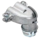
90° fitting with steel cover used to connect AC/MC cable or flexible metal conduit to box or enclosure. Simply snap connector into electrical box! External spring steel locking tabs secures connector. Refer to the cable connector compatibility charts in the technical guide section for MCI-A and other cables. Patented Whipper-Snap design.
