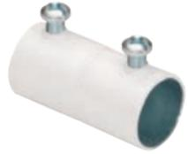
Set screw coupling used to join two lengths of EMT. Color coded white to match EMT for easy identification. Use with white EMT in light colored areas and open architecture applications. Concrete-tight. Furnished with Tri-Drive slot/Phillips/Robertson head screws. Patented.
