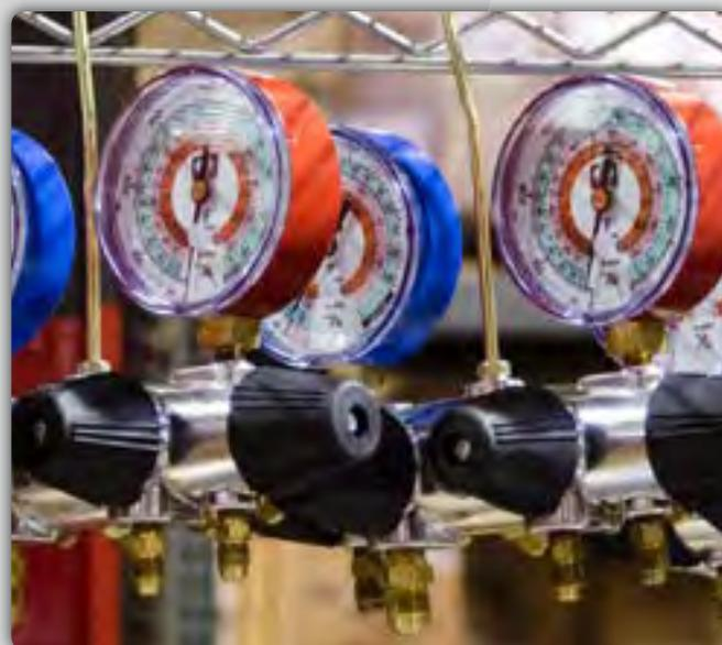
*Zeppelin manifolds are made from a single billet of solid aluminum*
