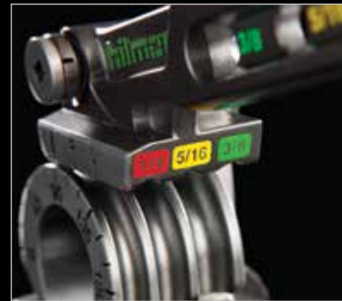
Correctly align the tube size with color-coded indicators.
