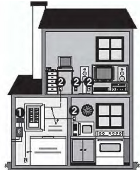
① CHSP installed at the service entrance panel. ② SurgeTrap™ surge traps and strips located where sensitive electronics are plugged in.
