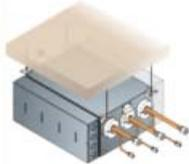
By reversing the electrical box position you can orient the inlet and outlet pipes into a left hand or right hand configuration.
