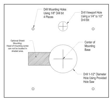
Head of mounting screw **CAN NOT** be located in shaded area
