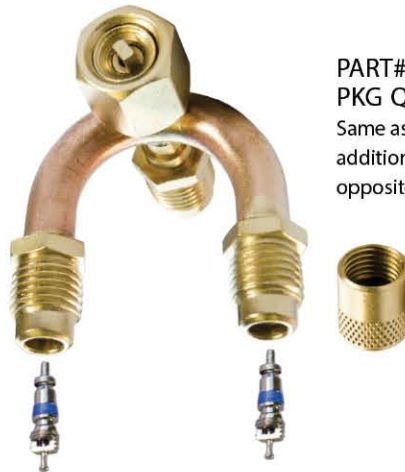
PART# CD2595 PKG QTY: 2 The same as CD2594, only the end of the copper tube opposite the female flare has been swaged to allow 1/4" copper tube inserted for brazing.
