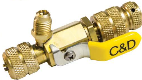
CD3930 PKG QTY: 1 BV-CRT for 1/4" flare connections and has 1/4" male flare side access port.
