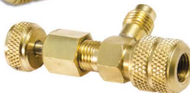
PART# CD2070 PKG QTY: 1 For 1/4" male flares. Depresses valve core and controls flow. Back seats and retains gas in the house.
