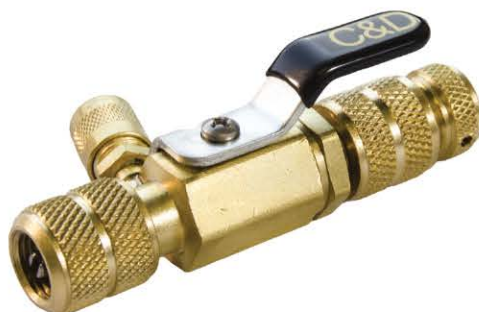
CD3956 PKG QTY: 1 BV-CRT for 5/16" flare connections and has 1/4" male flare side access port.
