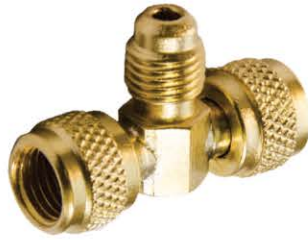
PART# CD2613 PKG QTY: 1 Two 1/4" female connections with o-ring seals and 1/4" male flare (without core) at right angle for connecting needs.
