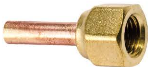
PART# CD2594 PKG QTY: 2 A 1-1/4" piece of 1/4" copper tubing, double flared on one end with a 1/4" female flare nut and a depressed tip.
