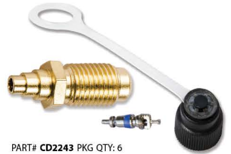
PART# CD2243 PKG QTY: 6 Flare length extended to 3/4", solder end - 1/8" ID, 3/16", 1/4", 5/16" OD steps (CD2217 cap)
