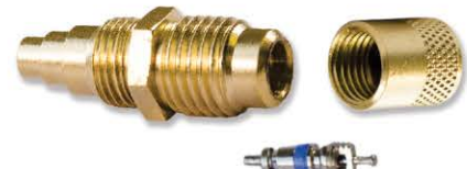
PART# CD3600 PKG QTY: 6 1/8" ID hole, 3/16", 1/4", 5/16", steps, 1/8" MPT below hex wrench cap and core
