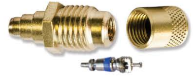
PART# CD8400 PKG QTY: 6 1/8" ID hole, 3/16", 1/4", 5/16" step, CD2245 cap and core
