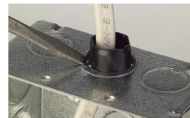
Easy Removal Push the wing tab of the connector with a screwdriver. Push the connector through the knockout towards the inside of the box.
