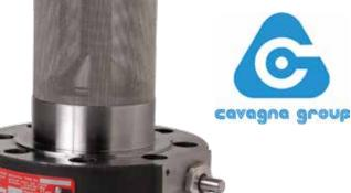
Cavagna flanged valves are equipped with a built-in excess flow to prevent the uncontrolled release of product. They are perfect for mounting a pump or piping direct to the internal valve. Mounting bolts are weakened allowing the pump or piping to "shear" in the case of an accident leaving the valve intact. Cavagna flanged internal valves have a filter to trap dirt and particles before entering the pump. This filter can be removed when the valve is installed on the filing pipe line.
