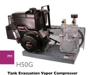
The Krug compressor transfers liquid by increasing vapor pressure in the tank being emptied, and decreasing vapor pressure on the tank being filled. A separate hose transfers the free flowing liquid.
