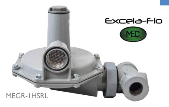
These light commercial second stage regulators are used to reduce outlet pressures from first stage regulators (normally 10 PSI) to 11"WC.
