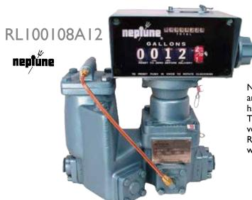
Note: 3/4" and I" meters are used in dispensers. Both have 3/4" FNPT flanges. The I" meter is the newer version with higher volumn. Read the data plate to verify which meter you have.
