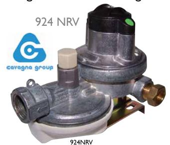
A combination of the first and second stage regulator which ensures a continuous flow of gas. The regulator automatically changes to the reserve tank when the first tank is empty. The indicator on the first-stage regulator changes from green to red to indicate the initial tank is empty.
