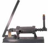
Simple piston hand pump for use in filling portable and motor fuel cylinders. Six gallon capacity at 40 strokes per minute.
