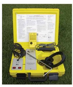
Cable Hound Underground Cable and Pipe Locator
