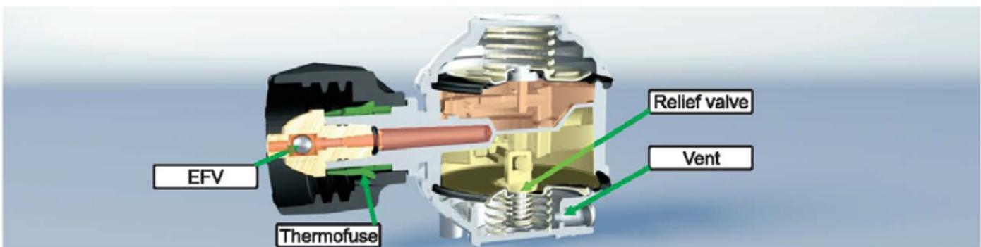
The gas tank pressure (from 25 to 250 PSI, red in the picture above) is reduced to 4 PSI by the first stage (orange in the picture). Then the second stage of regulation limits the pressure to 11 WC, final flow rate (yellow in the picture). The regulator is designed not to produce any sound vibration that may disturb the end user, whichever pressure the gas tank has got.
