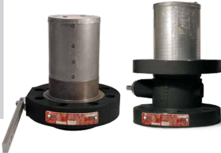
Cavagna flanged valves, equipped with a built-in excess flow valve to prevent uncontrolled product release, are perfect for mounting a pump or other similar piping connections.
