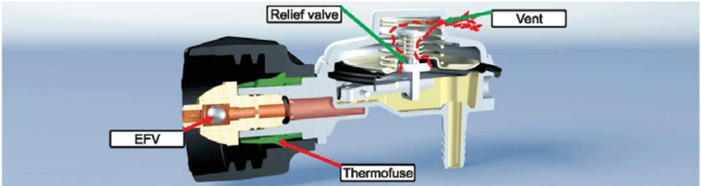
The gas tank pressure (from 25 to 250 PSI, red in the above picture) is regulated at 11 WC (yellow in the picture), the working pressure value for the gas appliances.
