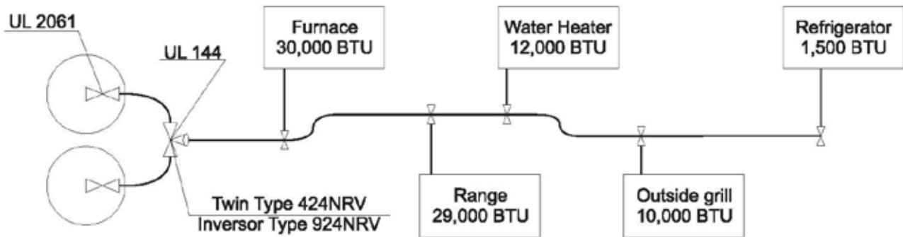
RV installations can be made on the basis of the following general diagram:
