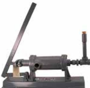
Simple piston hand pump for use in filling portable and motor fuel cylinders. Six gallon capacity at 40 strokes per minute.
