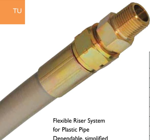
Flexible Riser System for Plastic Pipe Dependable, simplified compression style anodized service head. Reusable fitting with Buna seal, strengthened with a spiral steel stiffener. Integral swivel for easy installation. Complete with poly liner and lower moisture seal. Meets or exceeds NFPA58 and ANSI standards.. Available with 1/2", 3/4" MPT or 1/2" female flare service head, in 3', 6', 8' & 12' lengths.
