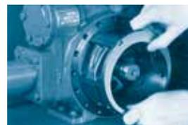
Easily replaceable liner restores efficiency.
