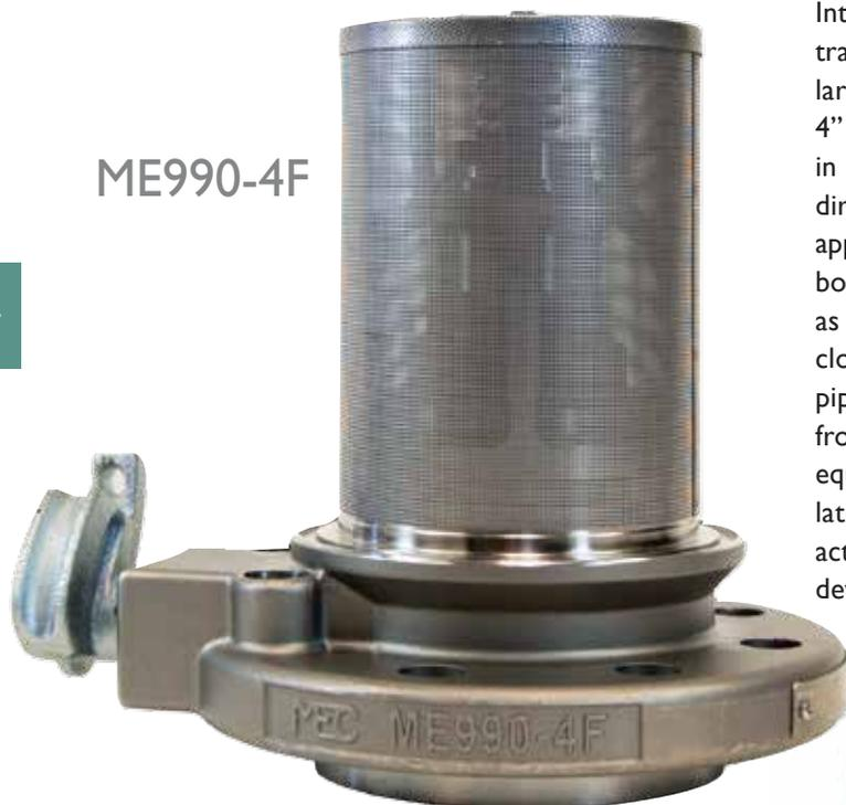
Intended for use on transport trucks and large storage tanks with 4" flanged connections in directional or bi-directional flow applications. Provides both manual shut-down as well as excess flow closing in the event of the piping being separated from the valve. Can be equipped with manual latch, pneumatic or rotary actuator open/ closing devices.
