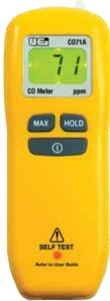
**CO71** ... Carbon Monoxide detector detects CO levels from 0 to 999 ppm. Tri-color warning indicates 3 concentration levels. Green when CO is 2-9 ppm. Amber when CO is 10-35 ppm and red with an audible alert at 34 ppm indicating dangerous CO levels. Handheld powered by 9V battery.
