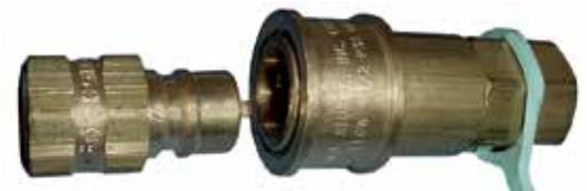
Quick Connect permits instant disconnection and fast, easy connection to gas supply line without using tools. Simply pull back operating ring and the coupling springs apart and shuts off gas. For gas connection bring two parts together until they snap in place. Fusible link (thermal shutoff) cuts off gas flow in presence of fire.
