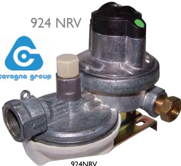
A combination of the first and second stage regulator which ensures a continuous flow of gas. The regulator automatically changes to the reserve tank when the first tank is empty. The indicator on the first-stage regulator changes from green to red to indicate the initial tank is empty.
