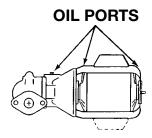
**NOTE:** The position of the conduit box is determined by the model of the motor used. The oiling ports must always be in the up position.
