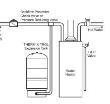
Stainless Steel System Connection. Maximum Operating Temperature: 200°F. Maximum Working Pressure: 150 psig Factory Precharge: 50 psig.
