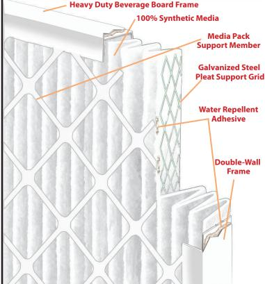
All Hi-E 40 filters are designed with a consistent pleat shape on predetermined centers causing dirt to collect evenly over the entire surface of the media. Fully utilizing every square inch results in a slow steady rise in resistance for maximum dust holding capacity.
