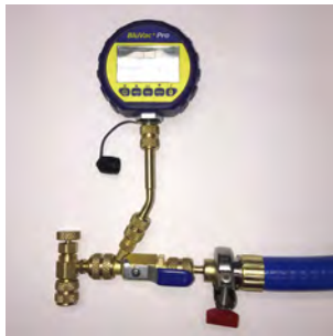
Core Tool with Vacuum Gauge Installed on Side Port and Schrader Core Depressor/Angle Valve
