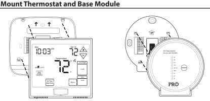
Align the 4 tabs on the subbase with corresponding slots on the back of the thermostat/base module, then push gently until it snaps in place.
