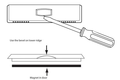
Gently slide a screwdriver into the bottom edge of the badge. Gently turn the screwdriver counter clockwise. The badge is held on by a magnet in the well of the battery door. The badge should pry off easily. **DO NOT USE FORCE.**
