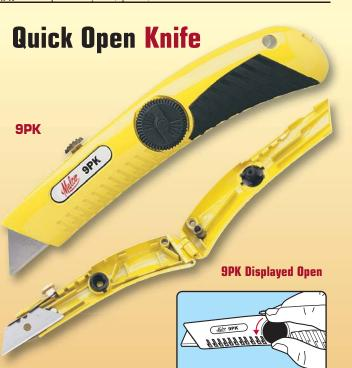
"No tools" blade change is fast and easy with just a turn of the knob. Extra blades store in handle. Retractable blade advances to 3 locked cutting positions with aid of thumb button. Heavy duty, die-cast knife halves feature "integrated hinge" to eliminate lost or dropped parts. Contoured knife shape features "ergonomic safety grip". One blade supplied in retracting mechanism.
