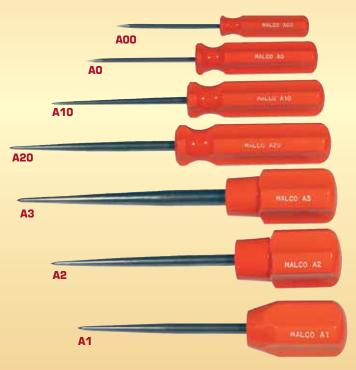
Use to scribe lines on metal, plastic and a variety of other materials. Pierce holes in wood, plastic, leather, - even light gauge metal. Blades are high carbon, alloy tool steel fully polished to resist rust. Blade tapers to a fine point and may be resharpened many times. Easy-to-spot orange handles are shock and shatter resistant. Shallow fluted handles with large end bearing surface provide a sure, comfortable grip. User has choice of large diameter or regular grip handles.
