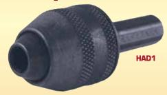
Accepts 1/4" hex power bits. Installs into chuck of a standard 3/8" power drill. Hex power bits can then be inserted or removed instantly without a key, by retracting the adapter sleeve. Tempered steel. Black finish.
