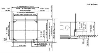
· Refrigerant piping and drain piping positions
