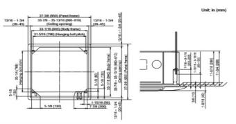
· Refrigerant piping and drain piping positions
