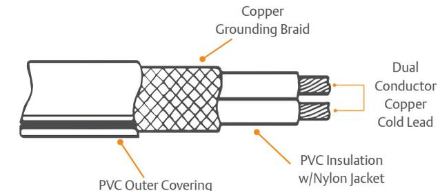
Cold Lead Dimensions: #14 AWG — 0.350 in x 220 in x 10 ft (8.89 mm x 5588 mm x 3 m)
