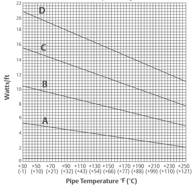
A HSR51F HSR52F    B HSR101F HSR102F    C HSR151F HSR152F    D HSR201F HSR202F
