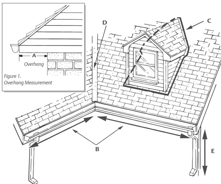
Figure 2. Roof Measurements
