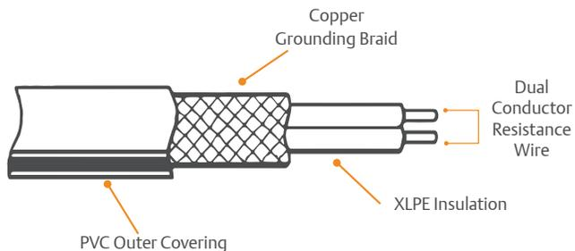
Heater Wire Dimensions 0.260 in x 0.165 in (6.604 mm x 4.191 mm)
