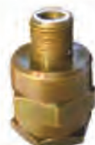
AFC-155 INLINE FILTER WITH MAGNET 1/4" FNPT Inlet 1/4" MNPT Outlet 12 Volt Cleanable and replaceable 40 micron filter element. Bonded ceramic magnet.
