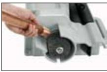
The optional Deburr Disk is used to grind the O.D. edge to help with tight fittings.
