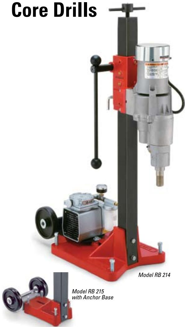
Ridge Tool offers two models of large capacity Core Drills. The RB214 is provided with a combination anchor/vacuum base which permits the user a choice of anchoring systems by incorporating the two types of systems in one base. The RB215 is ideal in that its base is designed solely for anchoring by masonry bolts.
