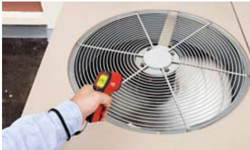
Measure efficiency of heat dissipation to reveal and locate thermal losses in the flow system.
