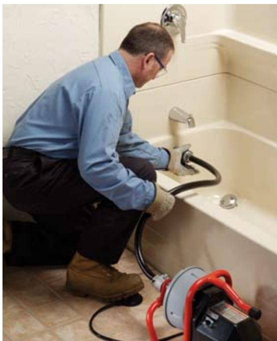
**In the tub:** Compact design allows easy access to hard-to-get-to areas like bathtubs and under-sink cabinets, while keeping the cable contained and away from all finished surfaces.
