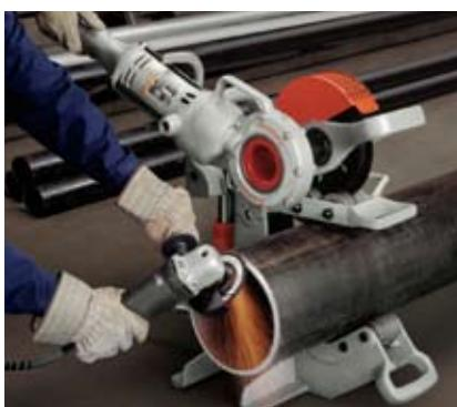
Model 258 with Pipe Roller in use for beveling.
