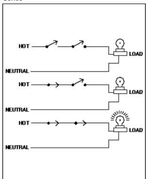
Both closed, circuit closed. One open, circuit open.
