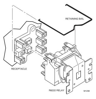
Fig. 9. Mounting relay to R8285J,K Relay receptacle.
