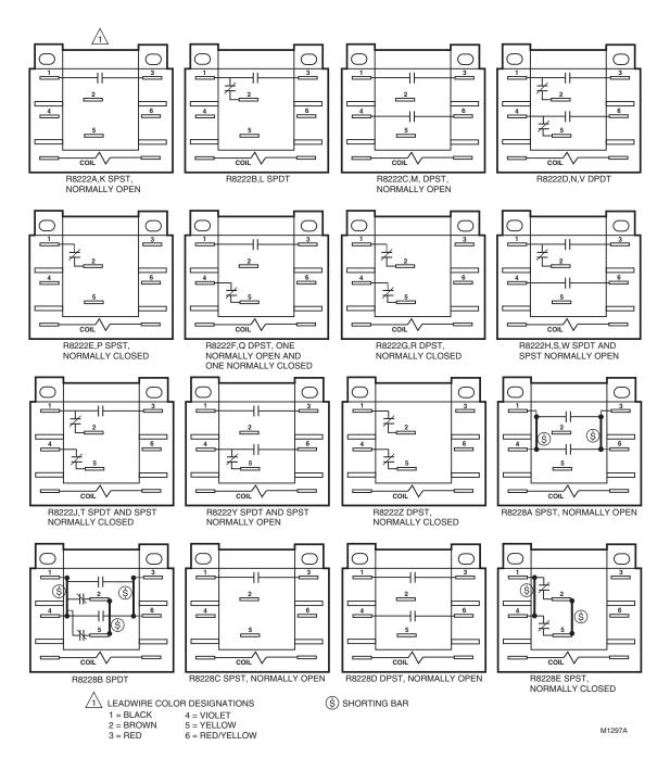
Fig. 7. R8285J,K Relay receptacle wiring diagrams with typical relays and applications.
