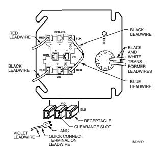
Fig. 8. R8285J,K Relay receptacle leadwire installation.
