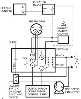
1 POWER SUPPLY. PROVIDE DISCONNECT MEANS AND OVERLOAD PROTECTION AS REQUIRED.
