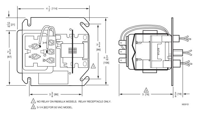
Fig. 1. R8285 installation dimensions in in. [mm].
