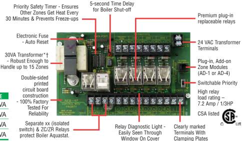
\* ARM-2P uses 20 VA Transformer. † Requires dry contact type thermostat or use of IR822 Isolation Relay
