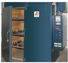
The development of **Pro-X 45000** ignitors followed a specific testing protocol to ensure they would be the toughest ignitors available. The design was validated by testing through hundreds of thousands of on/off cycles at high ambient temperature and maximum voltage.
